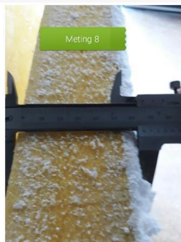
Set-up: 5 mm Power Acoustics 60 mm thick
