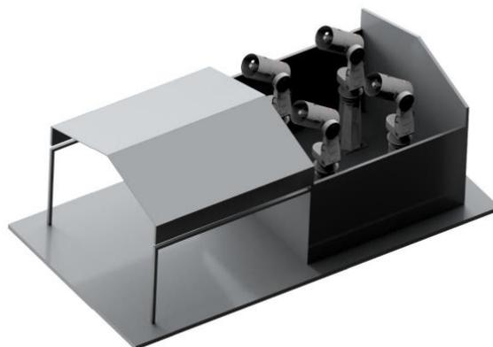
1.2 Automated Telescope Set (ATS) located at the Deep Sky Chile Observatory (South America / Chile) comprising a set of four ASA300UWF astrographs mounted on four independent PlaneWave L-350 direct drive mounts, cameras, custom air conditioning system, manufacturer's software (Sybilla Technology) with associated cabling and necessary hardware and accessories.
